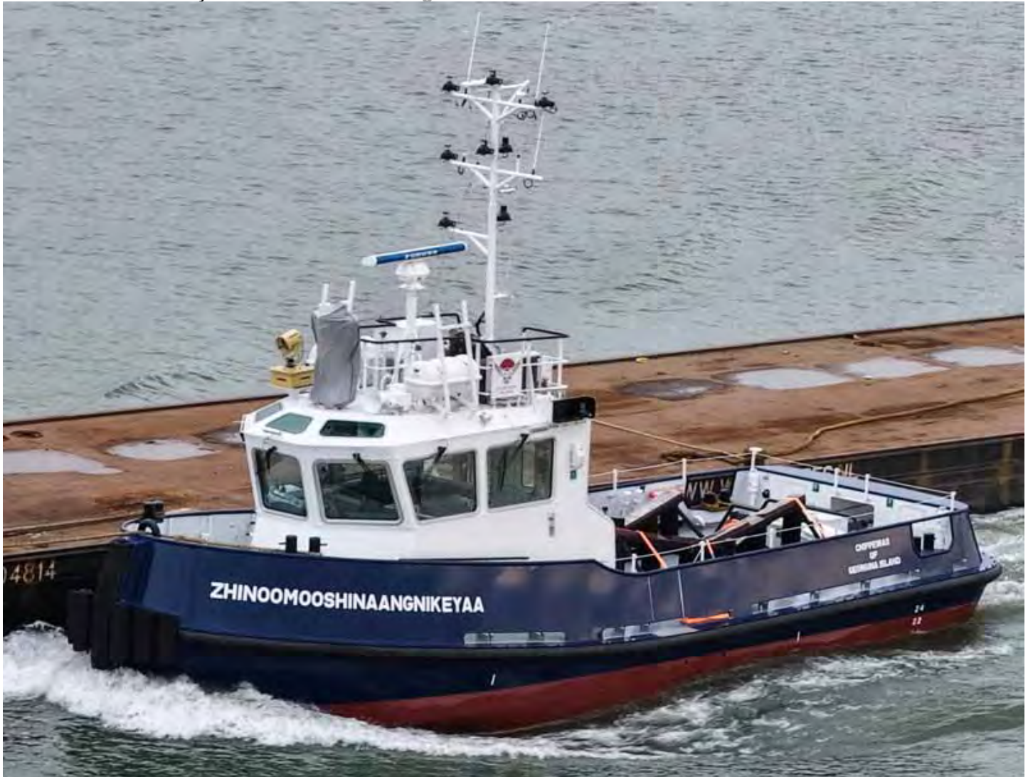
Damen build Stan Tug 1706 ice ZHIINOOMOOSHINAANGNIKEYAA enroute Antwerpen to be loaded on a Spliethoff cargo vessel to be transported to Canada. Photo : Arie Boer ©
